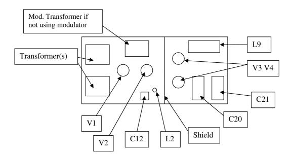
The crystal oscillator is some kind of Broadband, which means that any short wave crystal would work. The transmitter can easy modified by example for 76 meter. You only have to change the crystal, C12 & L2 and C20, C21 & L9.
